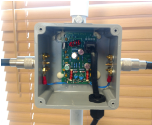
LNA mounted in box
