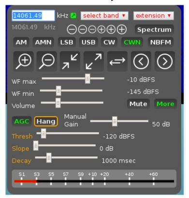
Generally for SSB I've found settings of 100 for Threshold, 3 for slope, and 1000 for decay, yield good results. CW probably works best with 130 for Threshold, 1 for slope, and 350 for
